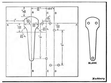
ig. 3. Lay-out of Die for Blanking and Piercing Stock as Illustrated in Fig. 2
